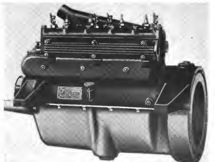
Valve side of the new Continental—the intake enters by means of a cored passage across the cylinder
